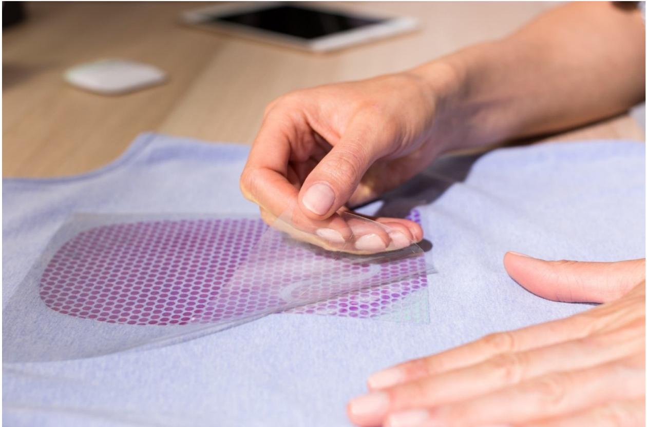
5. To free the second liner from your design, use your weeding tool to gently lift an edge away from the image. Then use your fingers to peel the liner from the image (warm peel).
